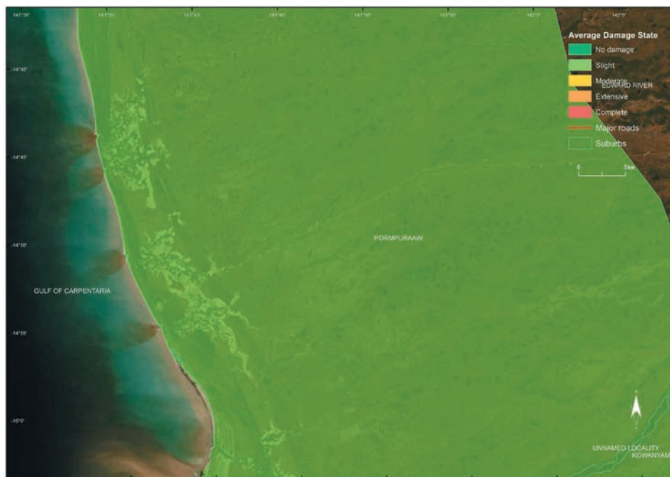
Figure 105: Aggregated residential building damage states for mesh block areas, for scenario 004-03396, a Category 5 cyclone impacting Pormpuraaw, Qld. Note that the spatial aggregation covers very large expanses in this part of Queensland, so any variation in damage within the community may not be discernible on this map.
